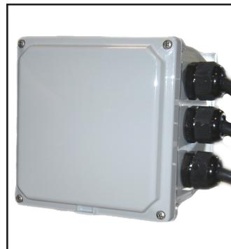
Cabling from each recloser module is terminated inside a junction box permitting a single cable to go to the control. Cable entry can be using either strain relief or twist lock style connectors.
